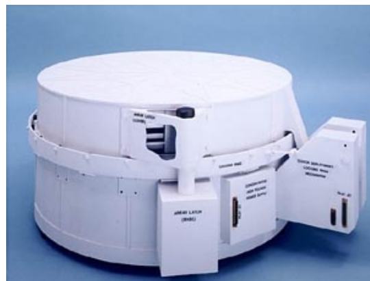
The Payload Canister contains wafers that collect solar wind particles.
